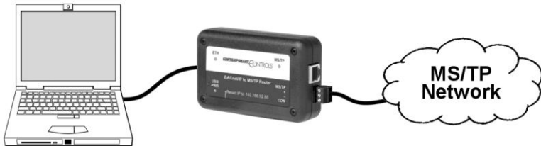
Figure 8 — Setup for Initial IP Address Configuration
