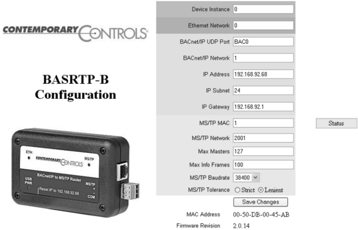
Figure 10 — Router Configuration Page with Default Values
