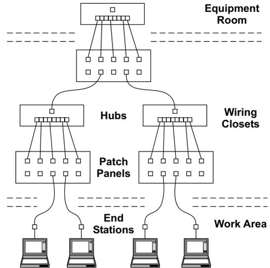
Figure 1. Structured wiring creates a hierarchy of hubs.
