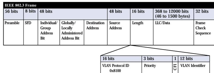
Figure 3. 802.1Q VLAN standard inserts a four-byte tag into a standard Ethernet frame.
