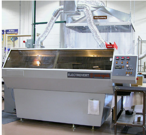
Another important step of the process for RoHS compliance was converting the company's solder wave machine by refitting pumps and changing solder pots to titanium.
