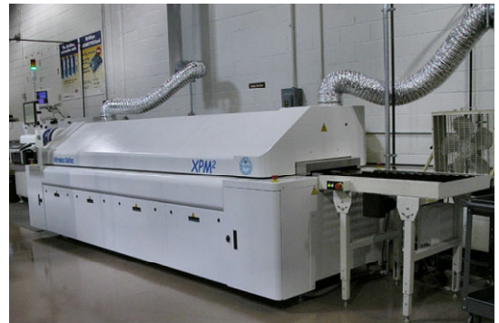
A new Vitronics® XPM820 reflow oven was purchased in order to solder at the required temperatures, necessary to meet RoHS compliance.
