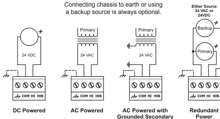
**WARNING:** Internally, this device utilizes a half-wave rectifier and therefore can only share the same AC power source with other half-wave rectified devices. Sharing a common DC power source is also possible. Sharing AC power with full-wave rectified devices is NOT recommended. Devices powered from a common AC source could be damaged if a mix of half-wave and full-wave rectified devices exists.
