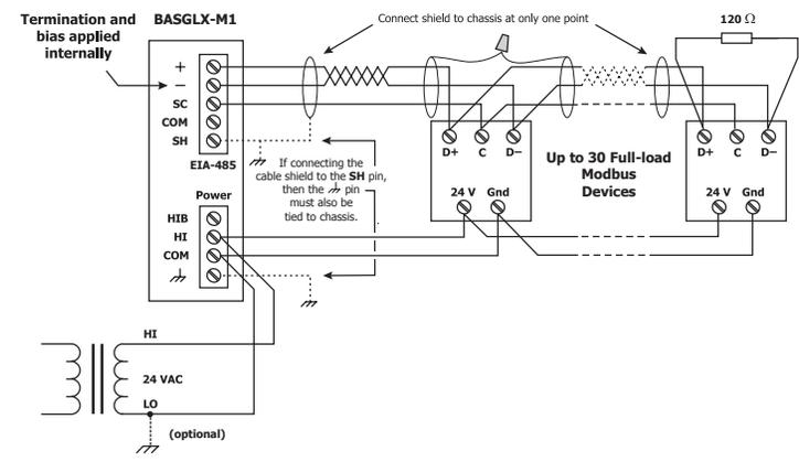
For Modbus devices that use a power source separate from the BASgatewayLX
