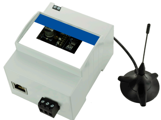
SBCti and hat in 4M enclosure for a wireless gateway
