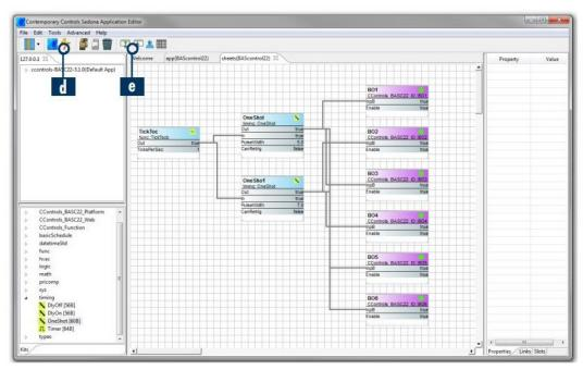
NOTE: The "Save to PC" and "Load from PC" buttons only save/load Sedona wire sheet applications. To save/load Sedona wire sheet and device configuration together as a single project file, use BASbackup.
