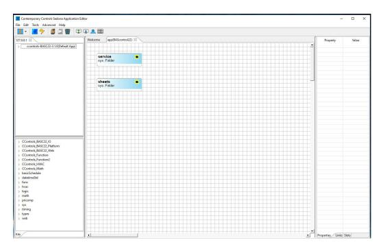
d. You are now connected to the BASemulator and you are ready to program function block diagram applications using SAE. To save your application, click the "Save to Controller' button. The saved wire sheet application will be stored in the emulator.
