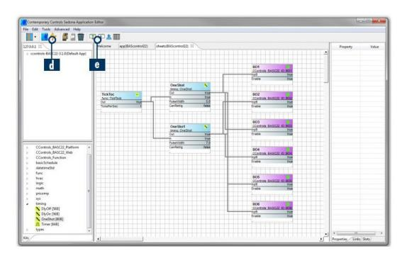
e. You may load an existing Sedona application (SAX file) using the "Load from PC" button at the toolbar in SAE. The emulated web page is able to reflect changes as the Sedona application is running. To observe current I/O channel response on the web page click the "Auto Refresh" button to "ON" state.
