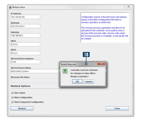
BASbackup is able to backup any BAScontrol with firmware 3.1.x or higher. To restore projects, the backed up project file must go onto a controller of equivalent or higher firmware version (from old to new). For example:
