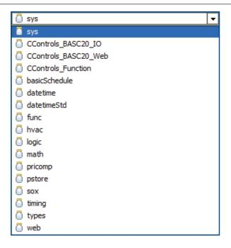
Using the drop-down, select the *CControls\_BASC20\_IO kit*. In the case of the BAScontrol20 there are 49 components to choose from – 20 real points, 24 virtual points, a scan timer and 4 retentive universal counters. All are intended for one time use and only those dragged onto the wire sheet will become part of the logic of the controller.
