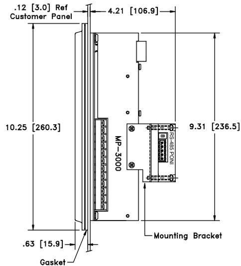
Figure 5: Mounting to an MP-3000
