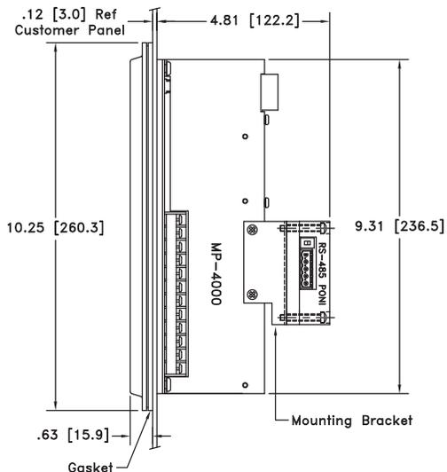
Figure 6: Mounting to an MP-4000
