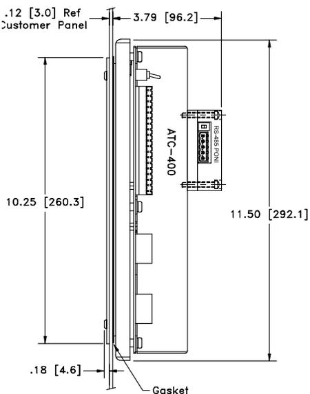
Figure 7: Mounting to an ATC-400
