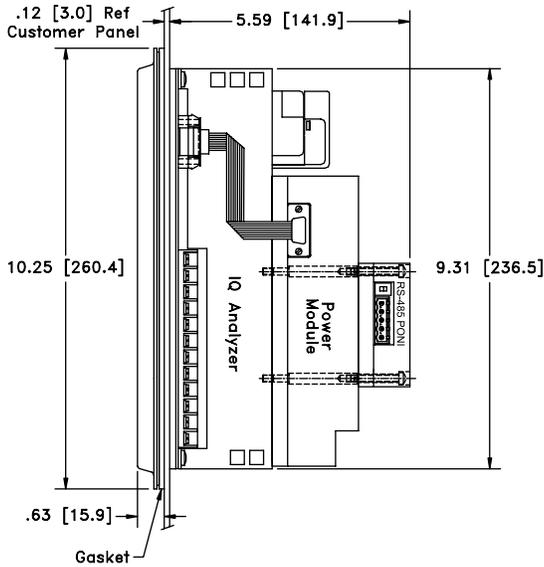
Figure 2: Mounting to an IQ Analyzer
