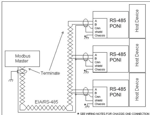
Figure 9. Typical RS-485 PONI Wiring Diagram
