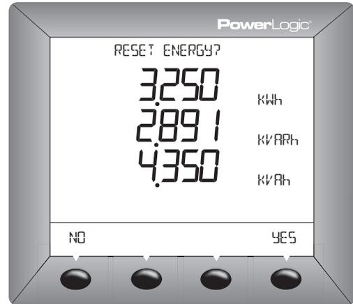
Individual settings for Demand, Min/Max, Mode, and Timer can be reset by selecting the value and using the above procedure.
