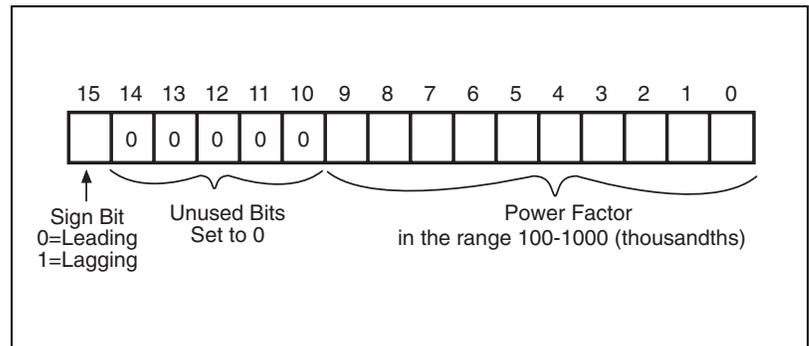
When the power factor is lagging, the power meter returns a high negative value—for example, -31,794. This happens because bit 15=1 (for example, the binary equivalent of -31,794 is 1000001111001110). To get a value in the range 0 to 1,000, you need to mask bit 15. You do this by adding 32,768 to the value. An example will help clarify.
