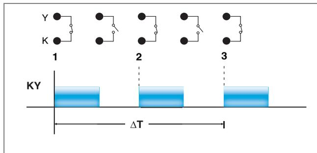
In Figure 5– 3, the off-to-on transitions of the output are marked as 1, 2, and 3. Each time the output transitions from off-to-on, the receiver counts a pulse. The power meter can deliver up to 8 pulses per second.
